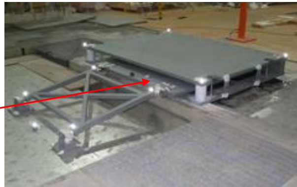
Figure 8. A full scale joint cover segment during shaking table tests at ENEA lab.
